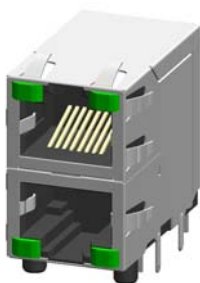
P/N RJ45-5385-02 SHOWN STACKED 2x1, 8 POSITION, WITH SHIELD AND LEDs
